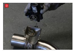
B) Lift up the motor. You will now be able to see the torsion spring (This must stay on the electronic valve motor to work with Scorpion Exhaust).
